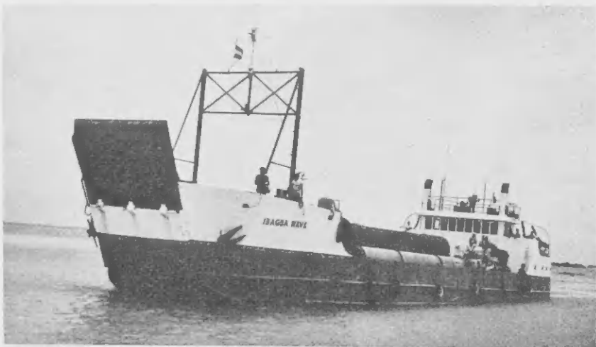
BY MEANS of the Pericles' heavy-duty long-reach boom, the converter is eased onto a special low-boy rig which rests on the deck of the landing craft. The base of the converter is supported on a separate set of wheels.
